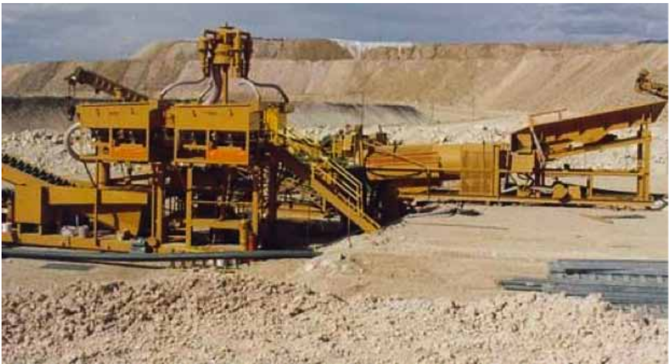
A 300 Yr 3 /hour capacity wash plant with a chemical final recovery circuit
